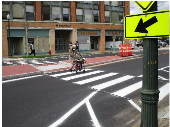
Photo 3: An improved crosswalk in Norwich. This crosswalk includes a median refuge and clear markings and signage. This is part of the award winning Franklin Square roundabout project , funded by the Community Connectivity Grant Program
